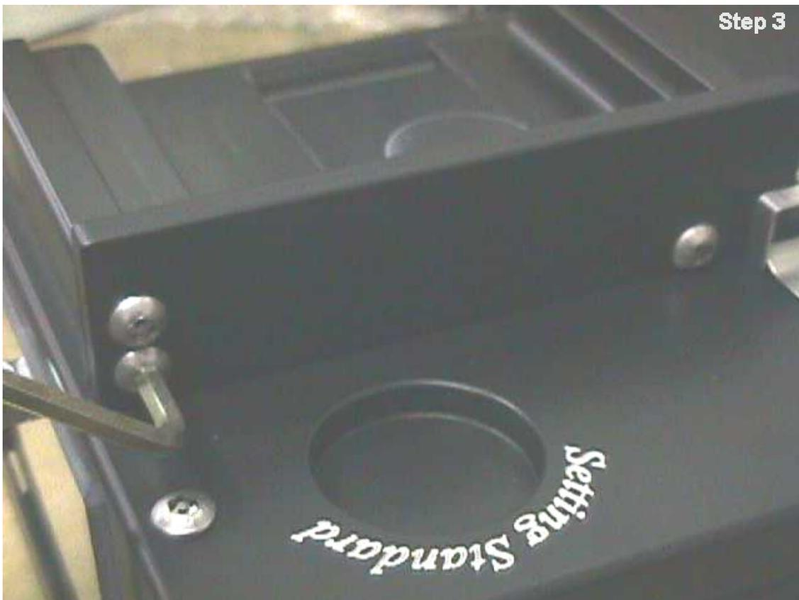
**STEP #3** – Remove the three button-head screws using the 5/32 security Allen wrench and remove the pocket guide. Next, completely remove the old tape.
