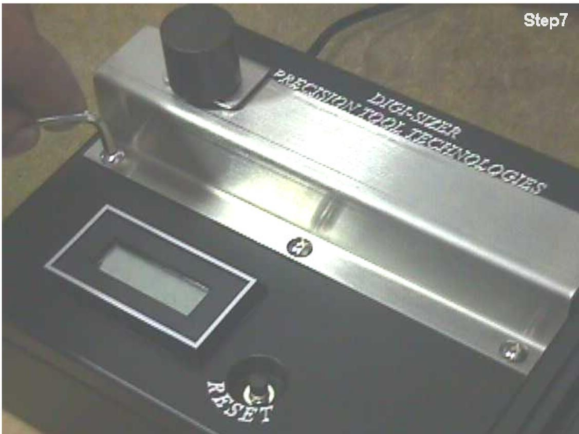
**STEP #7** – Put the front splash shield back on with the three bolts using the 5/32 security Allen wrench.
