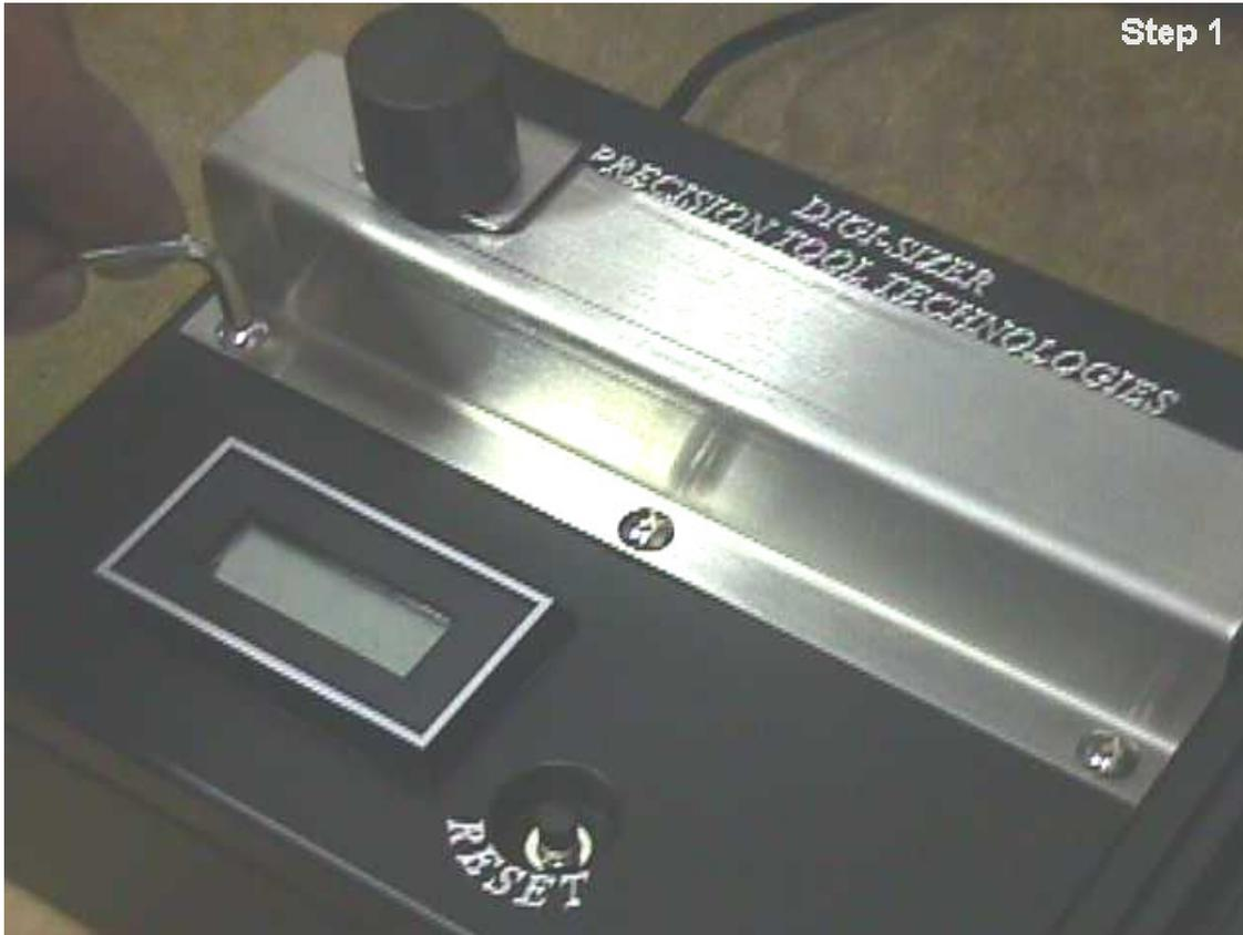
**STEP #1** – First remove the setting standard from its pocket, then remove the three button-head bolts from the front splash shield using the 5/32 security Allen wrench and remove the shield.
