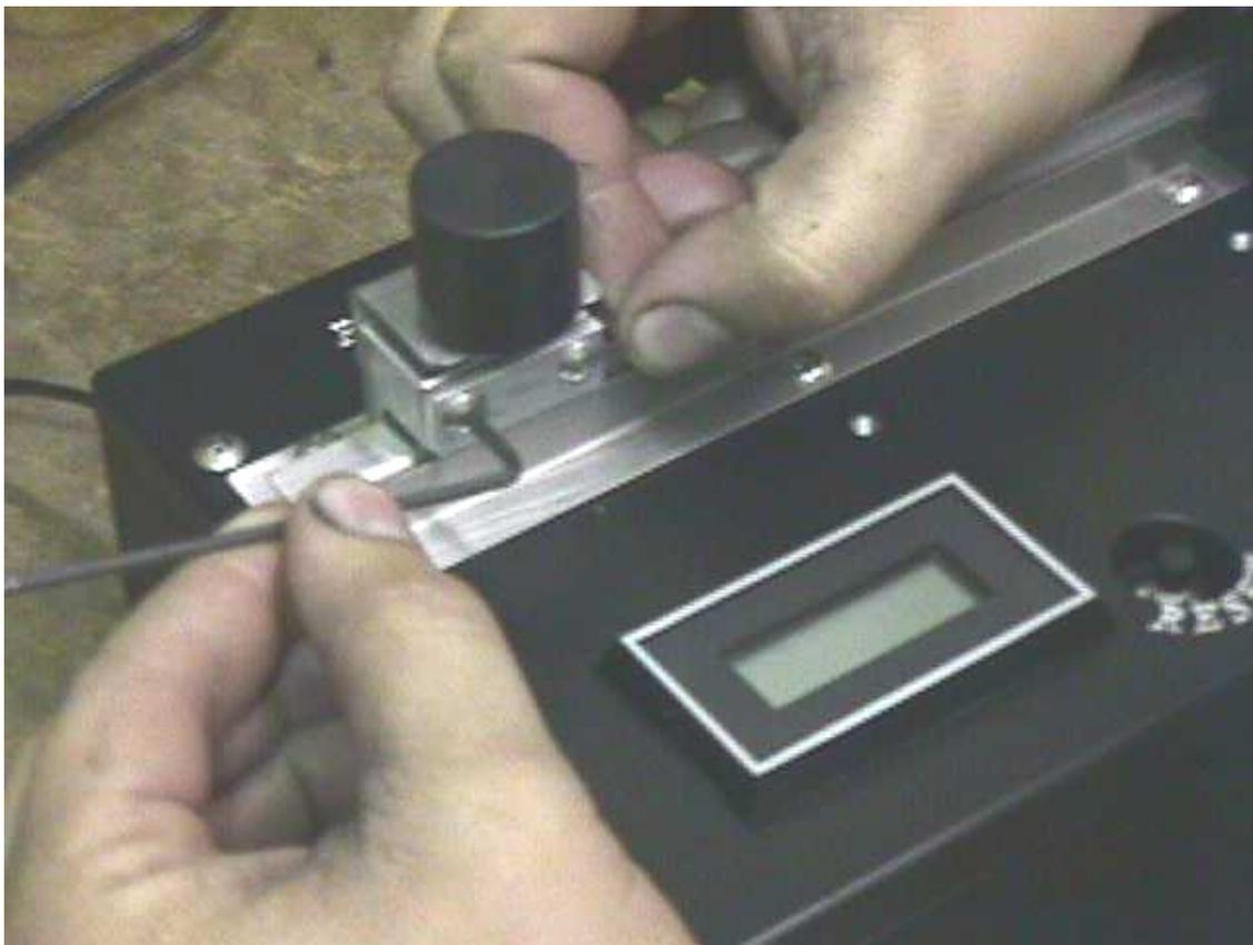
**STEP #5** – While holding the tape up against the step on the hidden side of the ribbon clamp and making sure the tape is all the way through the whole clamp, use the 3/32 Allen wrench to tighten the two button-head screws.
