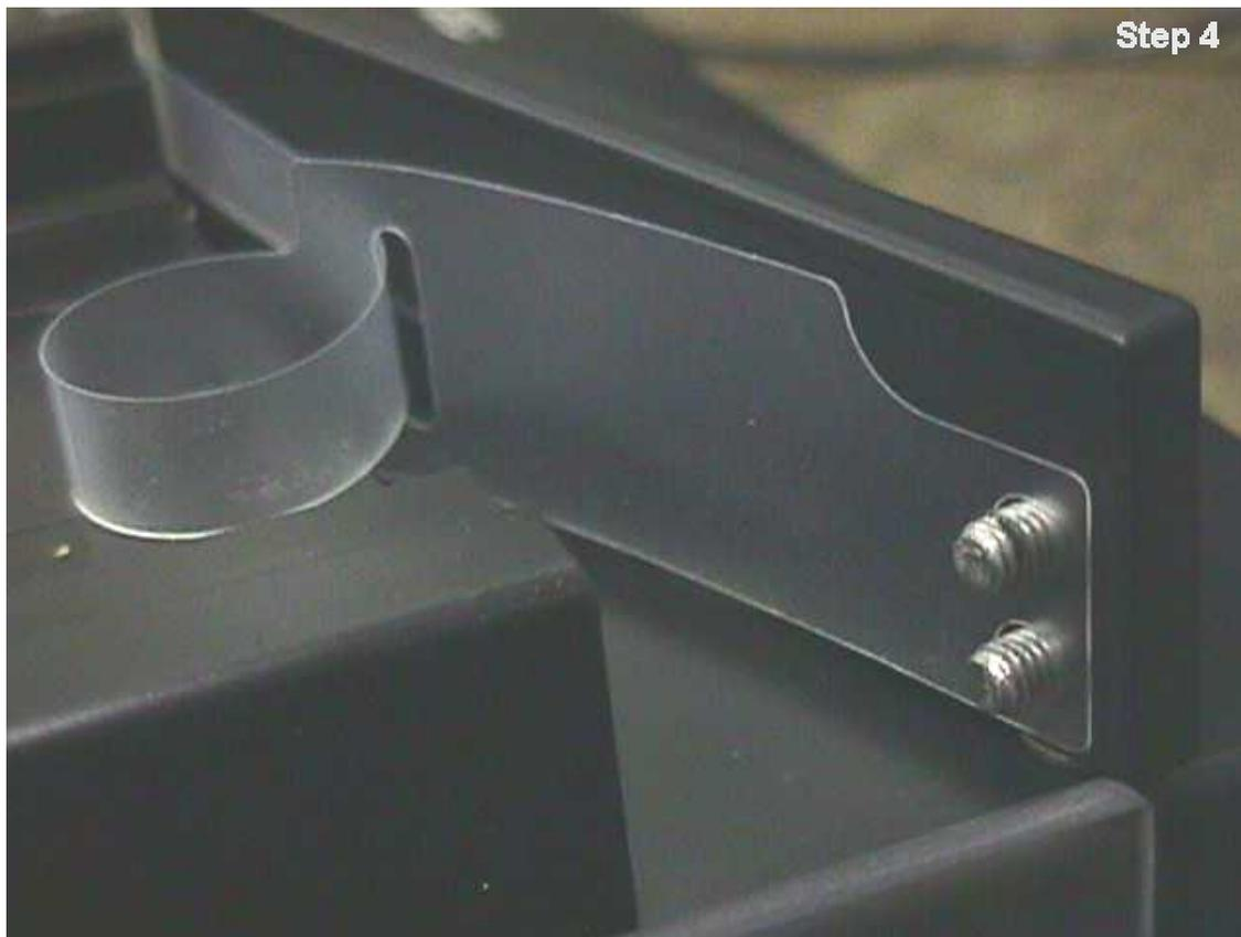
**STEP #4** –Replace with a new tape as shown in picture. Make sure tape is inserted correctly and the two tape holes go over the bolts. Then loop tape as shown in picture and snug the three button-head screws back into the pocket just tight enough so you can still adjust the tape.
